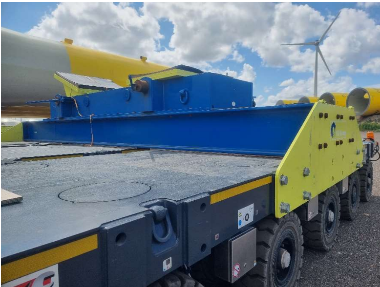
Figure 2, an adapter between SPMT and MP Transport Saddle
