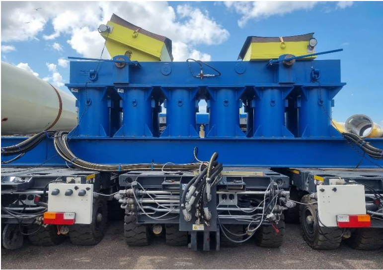
Figure 1, MP Transport Saddle with stools on SPMT
